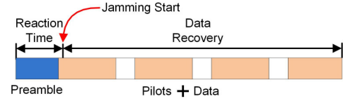
Fig. 5: Extended frame structure
